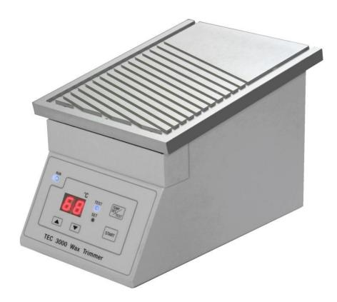
Wax Trimmer are a safe and practical instrument designed for removing excess paraffin from tissue cassettes following embedding. Simply slide paraffin blocks across the heated grooved plane surface, excess of paraffin is shaved away to disposable receptacle below.
